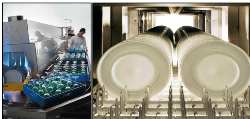
Figure 6-7: Principle of a rack conveyor dishwasher (left) and a conveyor-type dishwasher (right).
