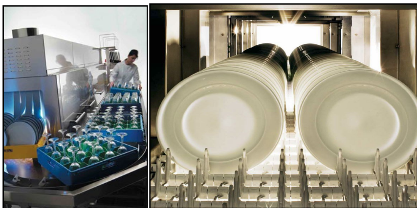
Figure 6-7: Principle of a basket conveyor dishwasher (left) and a belt conveyor dishwasher (right)
