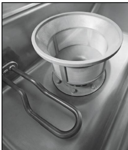
Figure 6-4: Filter and heating system of an undercounter one-tank dishwasher (category 2)
